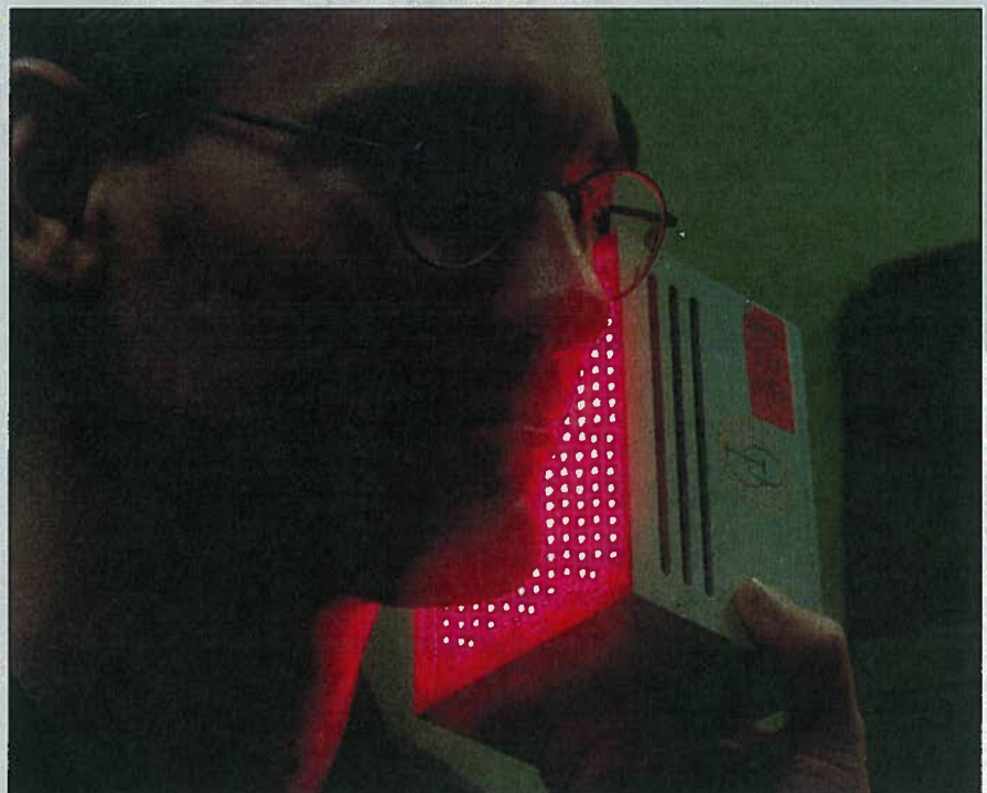
The wound-healing LED array device made by QDI is based on NASA-developed technology for plant growth. A nurse practitioner places the LED array on the outside of a patient's cheek, where it shines for just over a minute each day, promoting wound healing and preventing mouth sores caused by radiation and chemotherapy. (B. Himelhoch, Medical Center Graphics Inc.)
